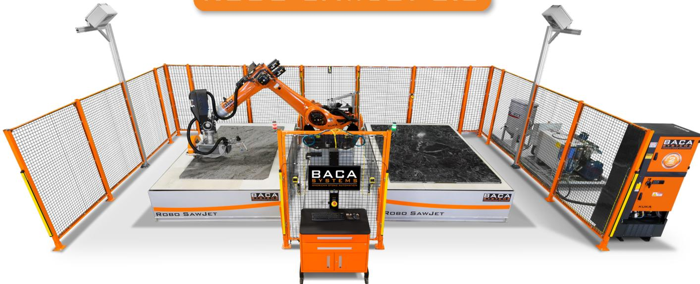
Adding a Robo SawJet to your fabrication process is the #1 way to increase profitability by reducing material cost by 10% to 15% through maximizing slab yield. In addition, Robo SawJet reduces the amount of downstream processing by reducing up to 4 hours of work on every slab by completing all arc cuts, radius cuts, sink openings and faucet holes during the sawing process. With an average cut time between 15-20 minutes per slab, you can let the saw complete 90% of your work.
