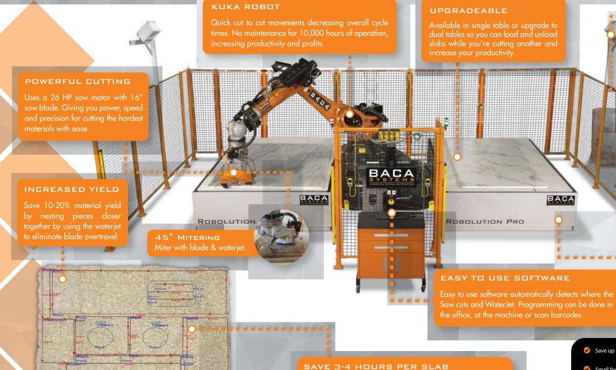
\*SAW USED TO MAXIMIZE SPEED \*WATERJET IS ONLY USED FOR NON-LINEAR CUTS & ELIMINATING BLADE OVERTRAVEL
