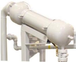
Water from the pit pump enters a centrifugal separator where solids are filtered to 40 microns. The Separators clean fluid provides the flush for the Pit Sweeper Package and is filtered further by a series of Hydro-Cyclones. Sludge from the Separator is deposited into a Sludge Hopper.
